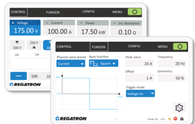
Figure 2: Intuitive control by HMI touch display. Everything you need at a glance.
